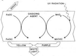
Deep purple-colored glass would be produced if the concentration of manganese in the melt was high and if strongly oxidizing conditions were present. It is conceivable that purple insulators were purposely produced for their beauty or for identifying or distinguishing different lines. The final color obtained with manganese present in the glass mixture (pinkish-purple to violet) would depend on such factors as
